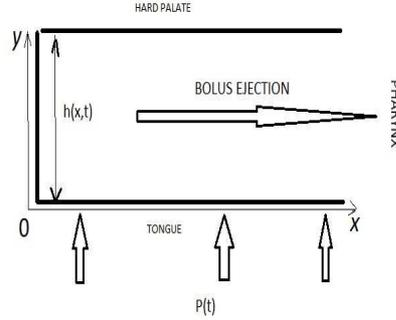
**Figure 2:** Diagram of a simplified model for oral stage bolus ejection. The movement of the tongue (bottom moving wall) is prescribed by either giving the height as a function of time and space,  $h(x,t)$ , or by specifying the pressure applied by the tongue as a function of time and/or space, i.e.  $P(t)$  or  $P(x;t)$  (the pressure applied by the tongue can depend on the  $x$  coordinate if the tongue is considered an elastic wall).
